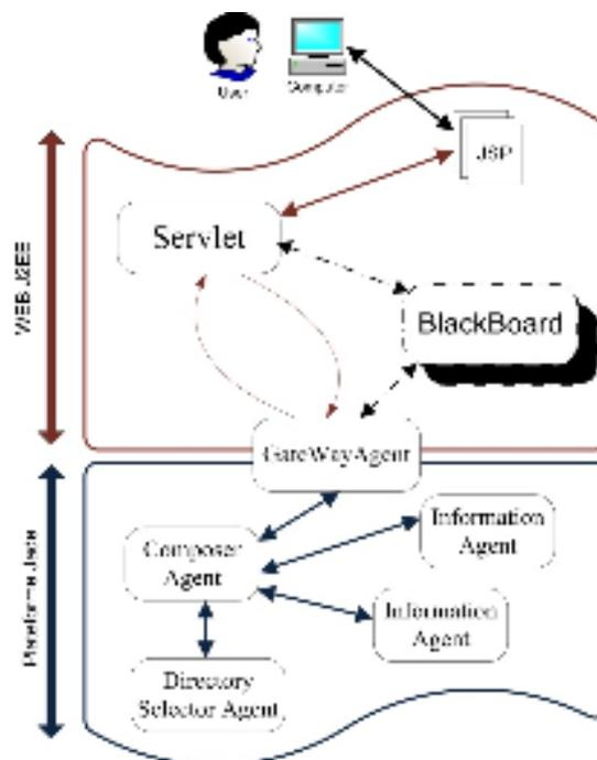
Fig. 5. The Servlet-agent architecture
