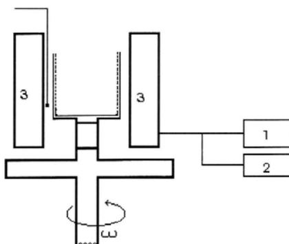
**Fig. 2.** The experimental device used for sedimentation on cylindrical surfaces. 1, 2- the electronic device for temperature and time setting. 3 – the oven
