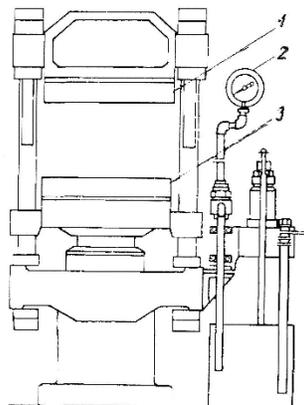
**Fig. 1.** The basic diagram of a hydraulic press: 1 -the upper plate, 2 - the manometer, 3 - the down plate
