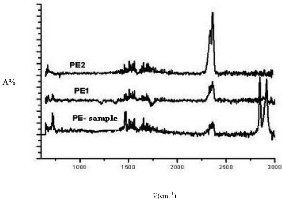
Fig. 4. The FT-IR spectra of PE-etalon, PE1 and PE2 films
