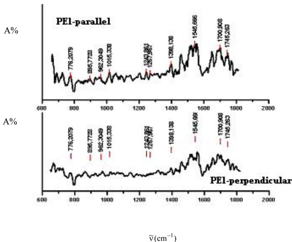
Fig. 3. The FT IR PE1- parallel and PE1-perpendicular spectra
