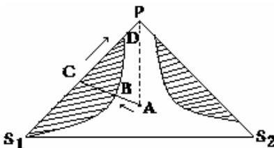
**Fig. 1.** The Scheme for obtaining the film polymer by the drying of a system with a polymer and two solvents
